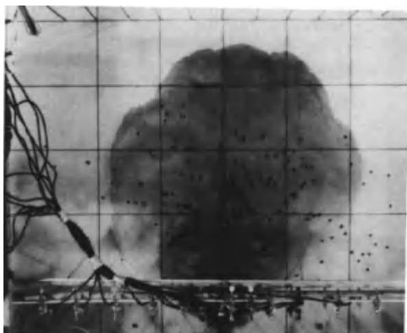
Figure 9.34 A horizontal buoyant jet with low momentum discharging into a laboratory flume (compare the jet with high momentum shown in Fig. 9.31). [Photo by B. Safaie.]
