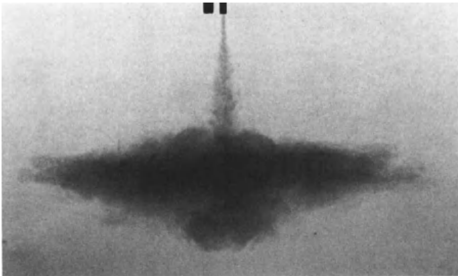
Figure 9.14 A vertical negatively buoyant jet descending in a stagnant, linearly stratified environment R_0 = 0.052 , N = 3.2 . [From Fan (1967).]
