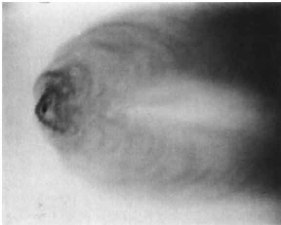
Figure 9.35 Laboratory model of flow shown in Fig. 9.30 made visible with colored dye. Note curved vortex seen upstream of the discharge point and plume bifurcation. Note also that dye intensity is not related to surface temperatures seen in Fig. 9.30.
