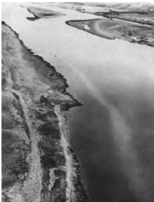
Figure 5.6 A plume resulting from a steady dye injection into the Columbia River near Hanford, Washington. (Photo courtesy of Battelle Northwest.)
